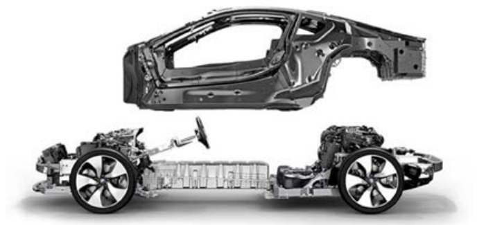
Carbon cabin and hybrid drive platform of the BMW i8
