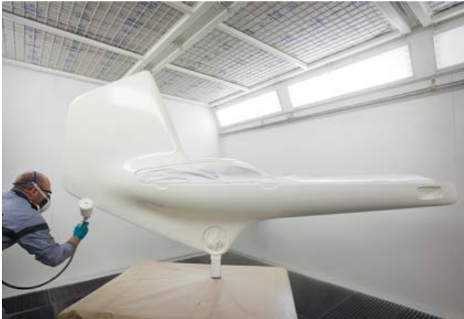
The bright color reveals all. The surface model on a scale of 1:3 being sprayed
