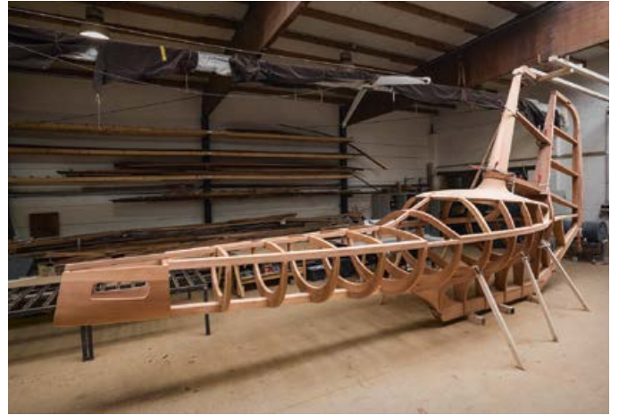
The mahogany frame model in its full size (10 metres long and 4.5 metres high) during the construction phase
